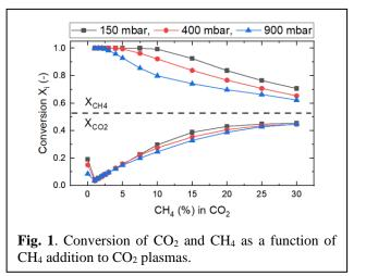
The afterglow model shows that hydrogen-containing radicals catalyse the recombination of CO and  $O_2$  for small CH<sub>4</sub> additions. Additionally, they are found to drive the water gas shift (WGS) reaction in the afterglow for higher methane additions (10-30%).
